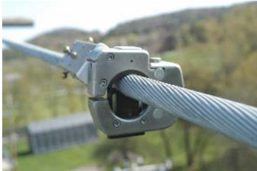
Figure 5-4 RF Conductor temperature and current sensor, offering power harvesting, live working install, and low cost. Cost is an order of magnitude lower than that of other available technologies.
