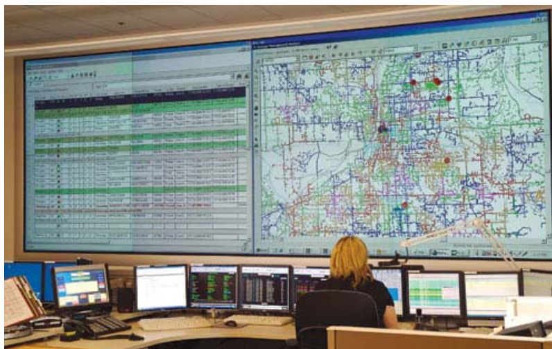
Figure 2. Example of a Visual Display from an Outage Management System
